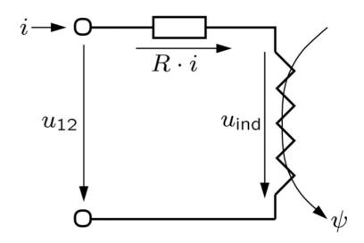
$\rightarrow$  Circuit parameters R,  $\psi$  computable from a suitable basis of the space of normal harmonic forms.
