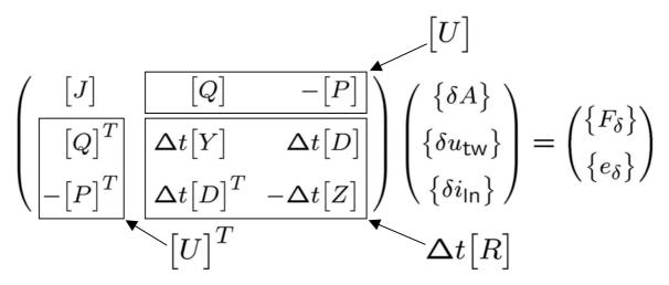
$\rightarrow$  Elimination of the circuit part [R] results in a s.p.d. Schur complement
