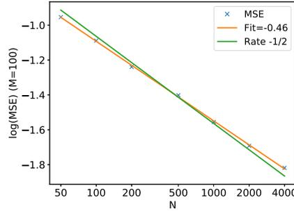
Fig. 8: Plot of the mean-square error MSE of (4.4) estimated for various values of  $N$  in logarithm scale for the case 3 of subsection 4.1.4. Using a least-squares regression, we find a convergence rate  $\text{Fit} = -0.46$ .
