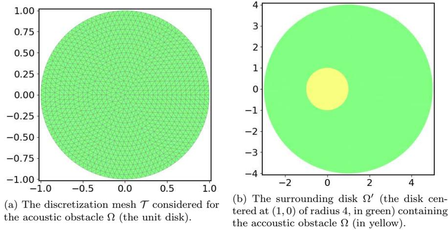
Fig. 10: Setting of the exterior acoustic problem (4.7): mesh of the circular acoustic obstacle  $\Omega$  and portion of the exterior domain  $\Omega'$  for the visualisation of the solution outside  $\Omega$ .
