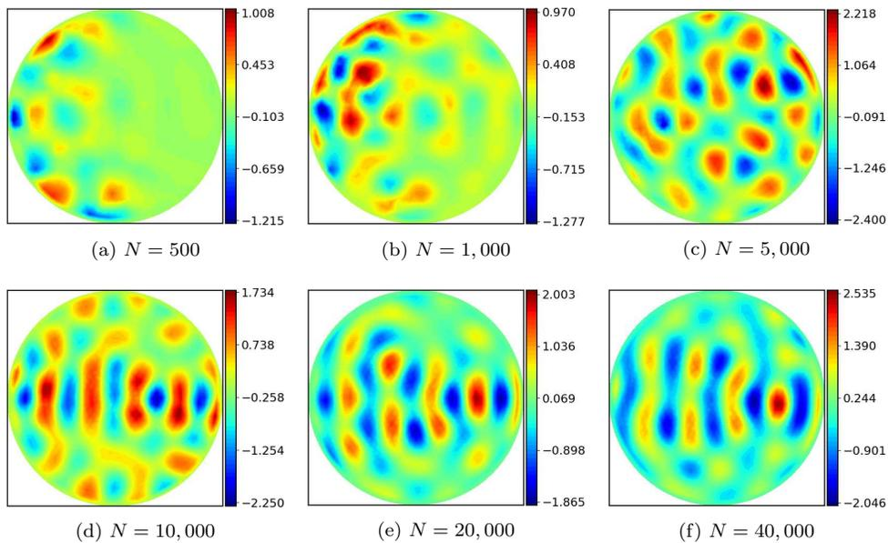
Fig. 13: Plots of Monte-Carlo solutions  $(z_i^p)_{1 \leq i \leq N}$  obtained by solving the linear system (4.9) for several values of  $N$ . The visualisation is obtained by using interpolated values on the triangle mesh  $\mathcal{T}$ .
