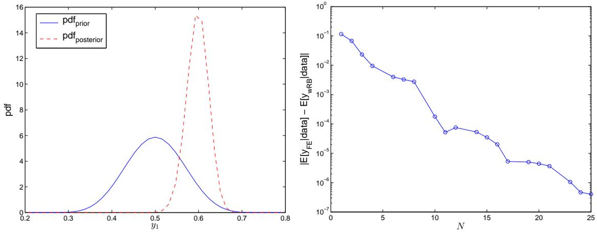
**Figure 9.** Left: the prior and the posterior density functions (pdf) of  $y_1$ ; right: decay of the weighted reduced basis approximation error for the expectation of  $y_1$  conditioned on the measurement data.
