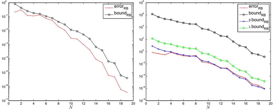
**Figure 11.** The error and error bound of reduced basis approximation of the solution of the Stokes problem (left) and for the Stokes optimal control problem (right).  $\beta$ : inf-sup constant;  $\lambda$ : regularization constant.
