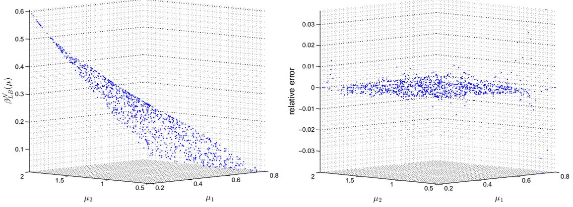
**Figure 2.** Dependence of the high-fidelity inf-sup constant  $\beta^N(\mu)$  on  $\mu = (m\mu_1, \mu_2)$  (left) and the relative approximation error of  $\beta^N(\mu)$  by Gaussian radial basis interpolation at 100 random samples (right).
