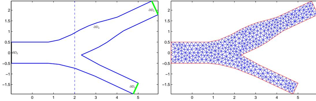
**Figure 10.** Left: sketch of a simplified geometry of the common carotid artery bifurcation (in 2d) and the cross section of the observation data (along the dashed line); right: a sample mesh of the geometry.
