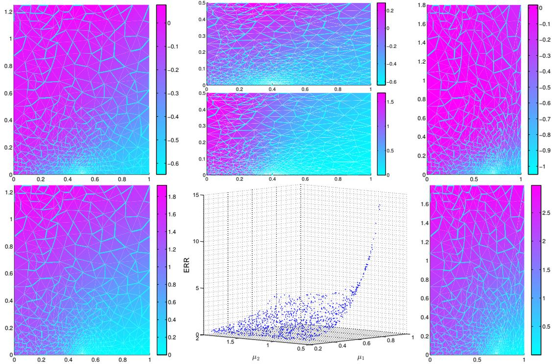
**Figure 3.** Left: displacement field  $u_1$  (top) and  $u_2$  (bottom) at  $\mu = (0.5, 1.25)$ ; middle:  $u_1$  and  $u_2$  (top) at  $\mu = (0.4, 0.5)$  and energy release rate (ERR) (bottom); right:  $u_1$  (top) and  $u_2$  (bottom) at  $\mu = (0.7, 1.8)$ .
