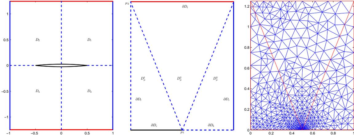
**Figure 1.** Left: geometry of a plate containing an internal center crack under tension, with four symmetric regions  $D_1$ – $D_4$ ; middle: the top-right region  $D_1$ ; right: an adapted/refined mesh near the crack tip region.
