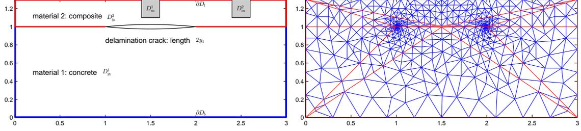
**Figure 6.** Left: the geometry of the material of composite and concrete with delamination crack in the interface and with two measurement sites; right: an adapted/refined mesh near the crack tip region.
