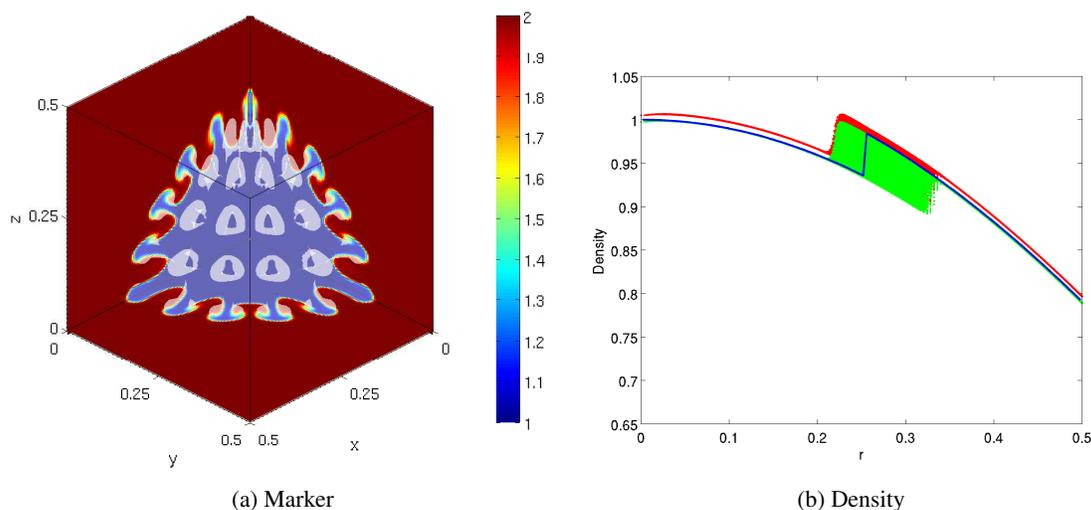
Figure 5: Rayleigh-Taylor instability within the three-dimensional polytrope.
