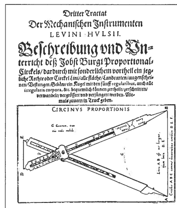
Fig. 3. Bürgi’s “Proportional Circkel”, a precision compass device invented and built by Jost Bürgi, first mentioned by Levin Hulsius in 1603 (published in 1607). It serves to reduce the scale of an object by a constant factor (from [19], p. 130).
