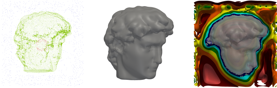
FIGURE 7. Left panel: Data points for the surface reconstruction. Red corresponds to a value of 1, green to a value of 0 and blue to a value of -1 . Middle panel: 0-level set of the posterior expectation evaluated at a regular grid. Right panel: Standard deviation for the reconstruction (blue is small, red is large).
