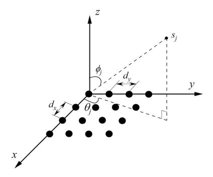
Figure 4.1: The geometry of a uniform rectangular array.
