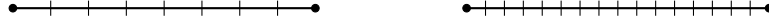
FIGURE 1. Two sets of equispaced nodes for a straight open arc. Dots represent fixed nodes, while dashes represent free nodes.
