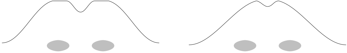
(a) Example of a mode for two coupled resonators. Observe that the mode is approximately constant inside both resonators.
