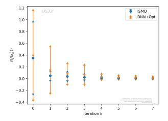
Figure 3: The objective function vs. number of iterations of the DNNopt and ISMO algorithms for the optimal control of projectile motion. The mean of the objective function and mean  $\pm$  standard deviation (3.16) are shown.
