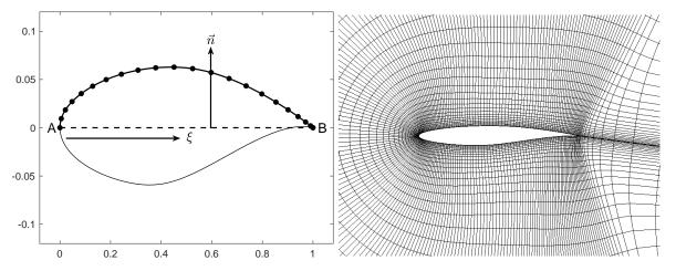
Figure 7: The reference shape of the RAE2822 airfoil. Left: The parametrization used to deform the shape of the airfoil according to (5.9). Right: The initial C-grid mesh used around the airfoil.
