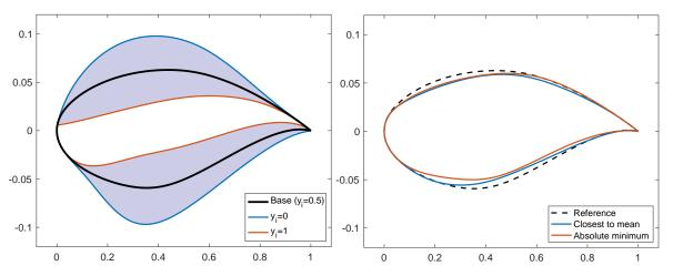
Figure 8: Shapes for the airfoil shape optimization problem. Left: The design envelope, where the reference, widest and narrowest airfoils are obtained by setting all design parameters  $y_i$  as 0.5, 0 and 1, respectively. Right: The optimized shapes obtained using the ISMO algorithm.
