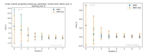
Figure 4: The objective function vs. number of iterations of the DNNopt and ISMO algorithms for the optimal control of projectile motion. The mean of the objective function and mean  $\pm$  standard deviation (3.16) are shown. Left: Random initial training points with  $N_0 = 8$  and  $\Delta N = 4$  for the ISMO algorithm. Right: Sobol initial training points for the ISMO algorithm with  $N_0 = 32$  and  $\Delta N = 16$ .
