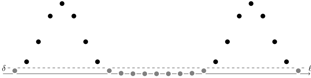
Figure 4: The function f_\lambda^+ from the introduction after discretisation. Entries of the resulting signal that fall below a certain threshold \delta > 0 are coloured in grey. The remaining entries are coloured in black and make up the vertex set V_\delta . In this picture, we can clearly see the two temporal islands.
