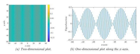
Figure 8: Real part of Bloch eigenfunction of the square lattice shown over many unit cells.
