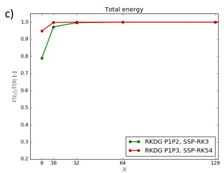
Fig 9a shows the electromagnetic energy after one periodic orbit as a function of number of zones along one direction of the two-dimensional mesh for P=1, P=2 and P=3 DG schemes. Fig. 9b shows the same information for P0P1, P0P2 and P0P3 schemes. Fig. 9c shows the same information for P1P2 and P1P3 schemes. All second order schemes are shown in blue; all third order schemes are shown in green; all fourth order schemes are shown in red.
