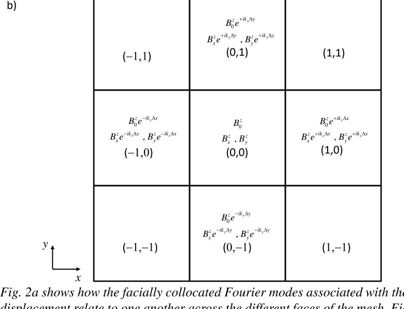
Fig. 2a shows how the facially collocated Fourier modes associated with the electric displacement relate to one another across the different faces of the mesh. Fig. 2b shows the analogous information for the Fourier modes associated with the magnetic induction. These Fourier modes are used in making the von Neumann stability analysis.
