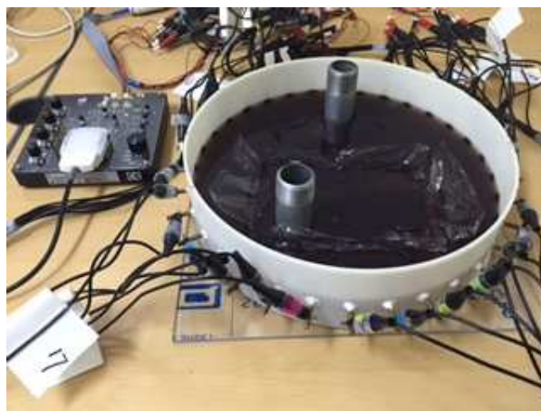
Figure 9. Configuration of phantom experiments by using Swisstom EIT-Pioneer Set.
