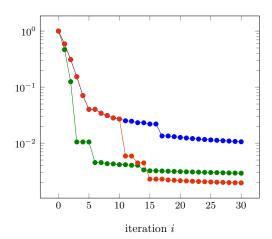
Figure 3: Evolution of the scaled absolute error (16) for a coarse (blue line) and a finer (green line) trial space  $V_N$ . Switching to a finer space after 10 iterations, it is possible start with a coarse trial space and still retrieve an approximate solution with good quality (red line).
