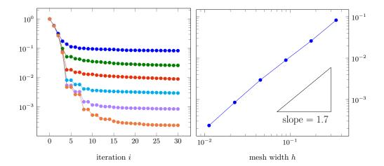
Figure 2: Left: Evolution of the scaled absolute error (16) on 6 nested meshes obtained with uniform refinement. Right: Value of scaled absolute error versus meshwidth at 30th iteration. We observe algebraic convergence with rate 1.7 (superconvergence).
