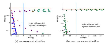
Fig. 6.3: Numerically computed open resonances found by an Arnoldi algorithm implemented in the hp finite element code NGSOLVE [2]. The different symbols stand for complex eigenvalues of (6.1), see [15] for more detailed explanations.
