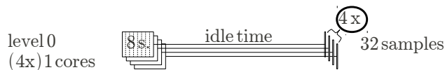
Figure 2: The “late save/4 tasks” strategy requests at least 4 tasks per level. In the example of Fig. 1 this leads to a large number of very small tasks on level 0.
