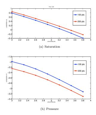
FIGURE 5. The difference in  $L^1$  between unregularized and regularized versions of the two-phase flow equations (2.1) with gravity. The plotted quantity is the log of  $\frac{1}{\mu}$  vs. the log of the relative error. Left: Saturation error and Right: Pressure. We consider solutions computed with the IMPES scheme on a  $100 \times 100$  and  $200 \times 200$  mesh.
