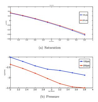
FIGURE 3. The difference in  $L^1$  between unregularized and regularized versions of the two-phase flow equations (2.1) without gravity. The plotted quantity is the log of  $\frac{1}{\mu}$  vs. the log of the relative error. Left: Saturation error and Right: Pressure. We consider solutions computed with the IMPES scheme on a  $100 \times 100$  and  $200 \times 200$  mesh.
