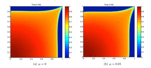
FIGURE 2. Solutions to the unregularized and regularized versions of the two-phase flow equations (2.1) without gravity. The plotted quantity is the saturation of water. Left:  $\mu=0$  and Right:  $\mu=0.01$  with  $\mu$  being the regularization parameter in (2.1). Both solutions are computed with the IMPES scheme on a  $200 \times 200$  mesh.
