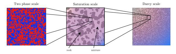
FIGURE 1. The three scales, in the middle scale one can define saturation.
