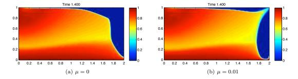
FIGURE 4. Solutions to the unregularized and regularized versions of the two-phase flow equations (2.1) with gravity. The plotted quantity is the saturation of water. Left:  $\mu=0$  and Right:  $\mu=0.01$  with  $\mu$  being the regularization parameter in (2.1). Both solutions are computed with the IMPES scheme on a 200 × 200 mesh.
