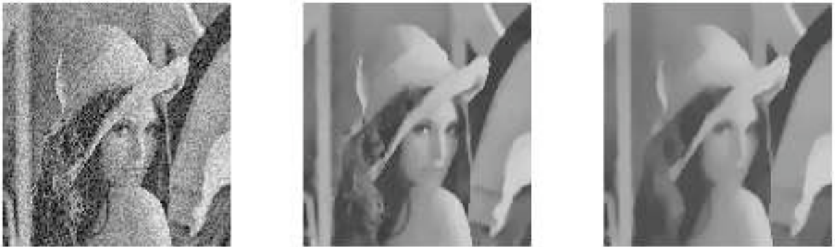
FIGURE 7. The initial noisy image and two smoothed samples at times t = 5 \cdot 10^{-4}, 10^{-3} using f_{\epsilon,2} -regularization. \epsilon = 10^{-5} , k = 10^{-5} , h = 2^{-8} and \lambda = 0 are used in the test.
