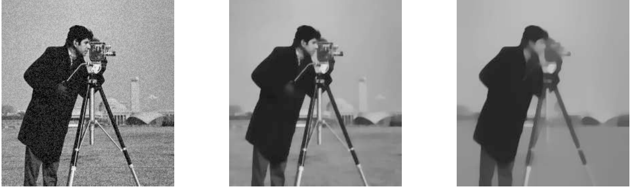
FIGURE 8. The initial noisy image and two smoothed samples at times t = 5 \cdot 10^{-4}, 10^{-3} using f_{\varepsilon,2} -regularization. \varepsilon = 10^{-5}, k = 10^{-5}, h = 2^{-8} and \lambda = 0 are used in the test.
