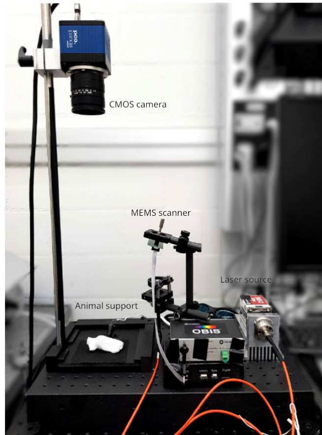
Figure 1: A snapshot of the latest stand-alone FMT hardware system in the animal imaging center of ETH Zurich. The main components of the hardware system include a sCMOS camera (detector), the animal support (object), the laser source and the MEMS scanner. Photo credit: Andrin G. C. Rickenbacher.
