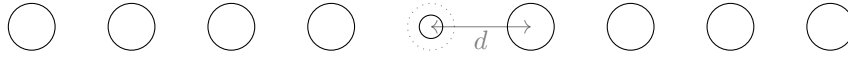
Figure 7: Two-dimensional cross-section of a finite subwavelength resonator chain with a point defect, which is expected to support an unprotected localized mode.
