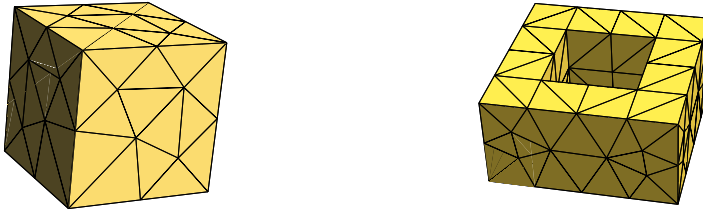
Figure 1. The two model geometries rendered with the coarsest triangular surface meshes used in the computations
