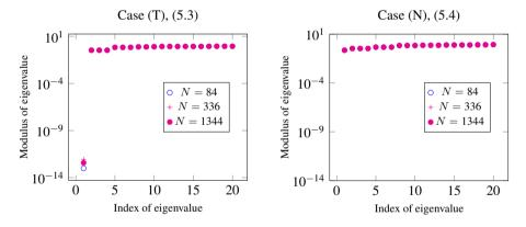
Figure 2. Cube: Plot of the 20 smallest approximate eigenvalues (in modulus) obtained by Galerkin boundary element discretization of (5.3) (left) and (5.4) (right) for different numbers N of flat triangles of the surface meshes.
