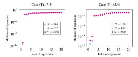
Figure 3. "Cubic doughnut": Plot of the 20 smallest approximate eigenvalues (in modulus) obtained by Galerkin boundary element discretization of (5.3) (left) and (5.4) (right) for different numbers N of flat triangles of the surface meshes. Discretization errors affect the eigenvalues more severely in the case (N), where the discrete kernel  $\operatorname{Ker}_h(\mathsf{b}_N)$  is not a subspace of the boundary element space and contains functions with strong edge singularities.
