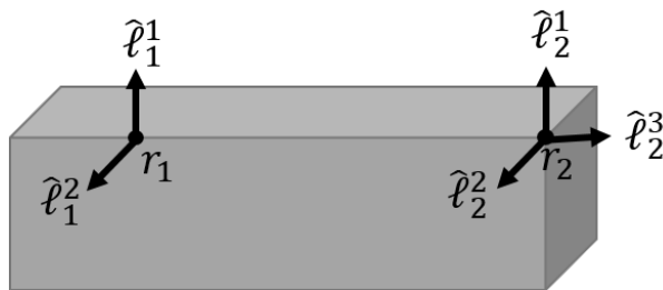
Figure 2. Directions of B-splines assigned to \mathbf{r}_1 and \mathbf{r}_2 located on an edge and on a corner, respectively.
