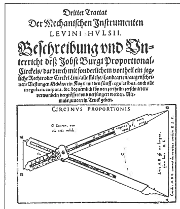
Fig. 3. Bürgi’s “Proportional Circkel”, a precision compass device invented and built by Jost Bürgi, first mentioned by Levin Hulsius in 1603 (published in 1607). It serves to reduce the scale of an object by a constant factor (from [17], p. 130).
