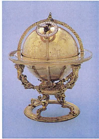
Fig. 2. The little “Himmelsglobus”, completed by Bürgi in 1594, to be seen in the Swiss National Museum in Zürich, see [12], [17]. It is an extraordinary piece of early astronomy and precision craftsmanship, 142 mm in diameter and 255 mm of total height, accurately displaying the motion of the celestial sphere, the sun, and giving the time.
