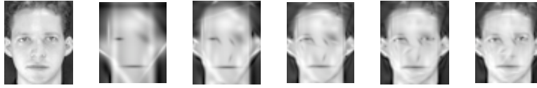
Fig. 4. Progressive OMP approximation of a human face (leftmost) with 20, 50, 80, 110 and 140 Gaussian atoms (from left to right).
