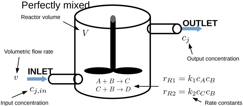
Continuously Stirred-Tank Reactor
