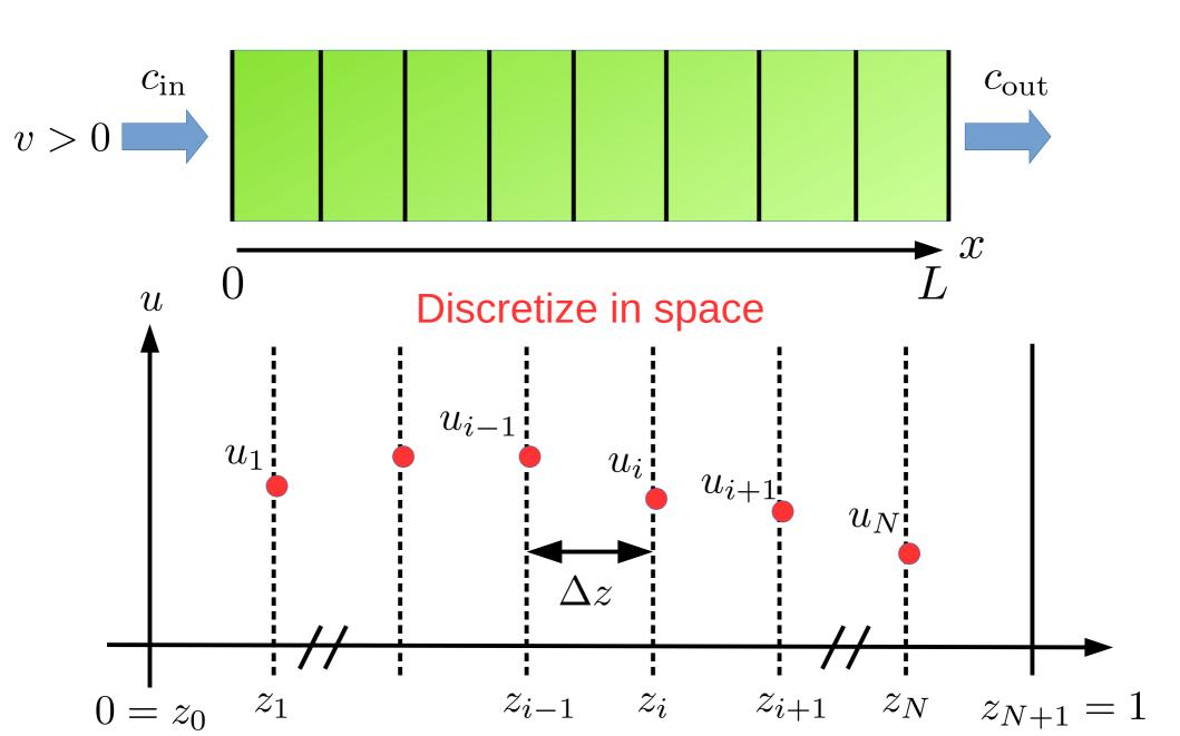
$$\frac{\partial u}{\partial \theta} = \frac{1}{Pe} \frac{\partial^2 u}{\partial z^2} - \frac{\partial u}{\partial z} - Da \cdot u^n$$
