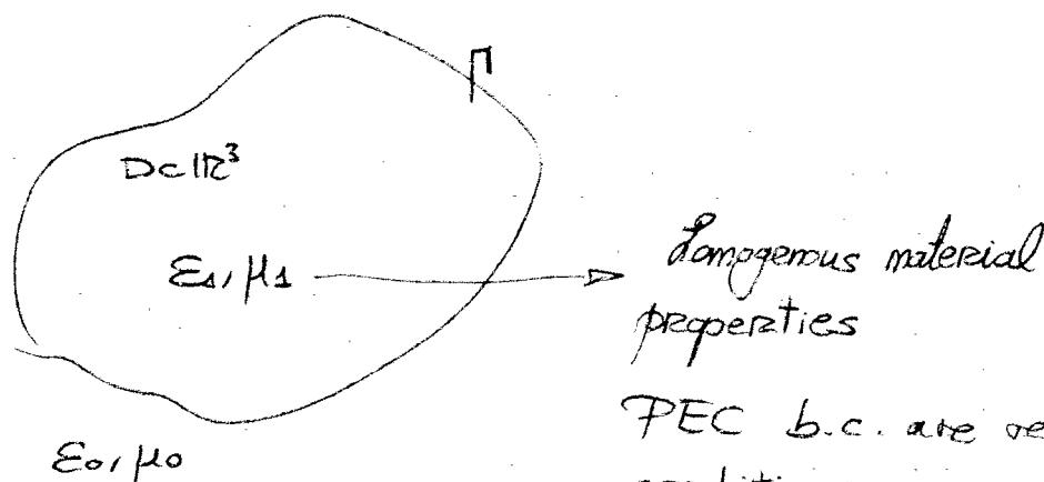
PEC b.c. are replaced by transmission conditions.
