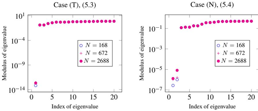
Figure 3. “Cubic doughnut”: Plot of the 20 smallest approximate eigenvalues (in modulus) obtained by Galerkin boundary element discretization of (5.3) (left) and (5.4) (right) for different numbers  $N$  of flat triangles of the surface meshes. Discretization errors affect the eigenvalues more severely in the case (N), where the discrete kernel  $\text{Ker}_h(\mathbf{b}_N)$  is not a subspace of the boundary element space and contains functions with strong edge singularities.
