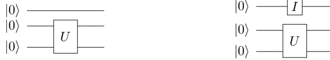
(a) Unitary gate and implicit identity gate. (b) Unitary gate and identity gate.
