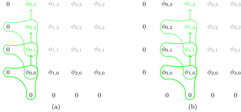
Figure 3.17: Second step in the efficient application of the recursion stencils in two dimensions. All values we initially know are printed in black. In a first step we centre the cheap stencil \mathcal{S}_1^2 at the node \underline{k} = (0, 0) and compute \phi_{0,1} only. Next we can use the same stencil centred at \phi_{0,1} and find \phi_{0,2} . We continue like this until an overflow occurs. (In this little example we are done after the next step.) Now we can start the second chain at the anchor (1, 0) and recursively compute \phi_{1,1} , \phi_{1,2} , \phi_{1,3} until the overflow occurs. In a next step (not shown here) we start a chain at (2, 0) , then at (3, 0) and so forth until the last node (k, 0) .
